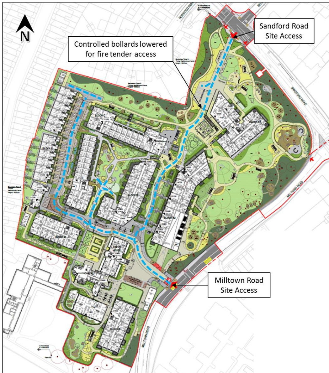
Figure 2.4: Fire Tender Access Route
