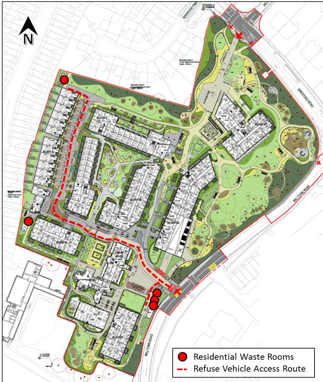
Figure 2.5: Surface Level Residential Waste Collection Areas
