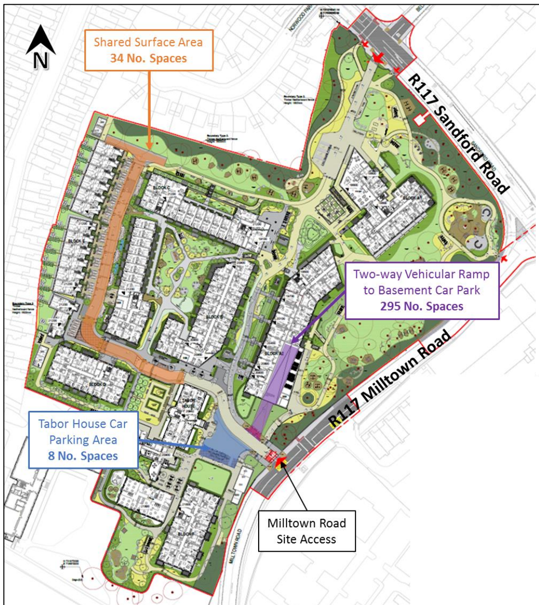
Figure 3.1: Vehicle Parking Areas Accessible via Milltown Road
