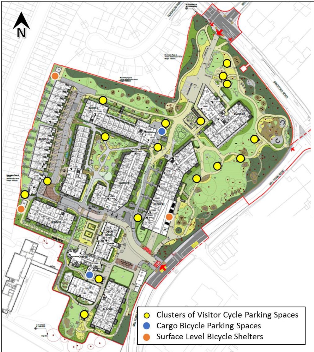
Figure 5.1: Bicycle Parking Layout at Surface Level
